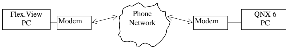
Fig. 2. Dial-up connection to a single RealFlex PC
