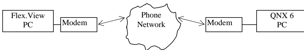
Fig. 2. Dial-up connection to a single RealFlex PC
