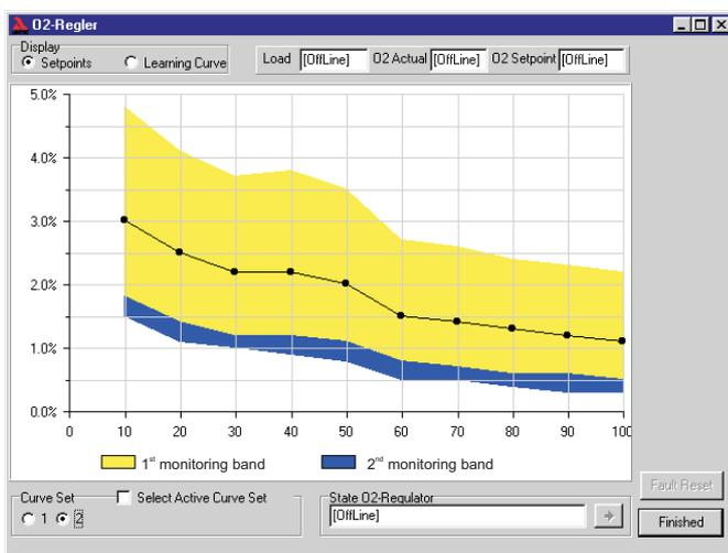
Fig. 4: Visualisation of the  $O_2$  setpoint-curve including monitoring-band-gaps when using the integrated  $O_2$  controller of the VMS and with remote control software
